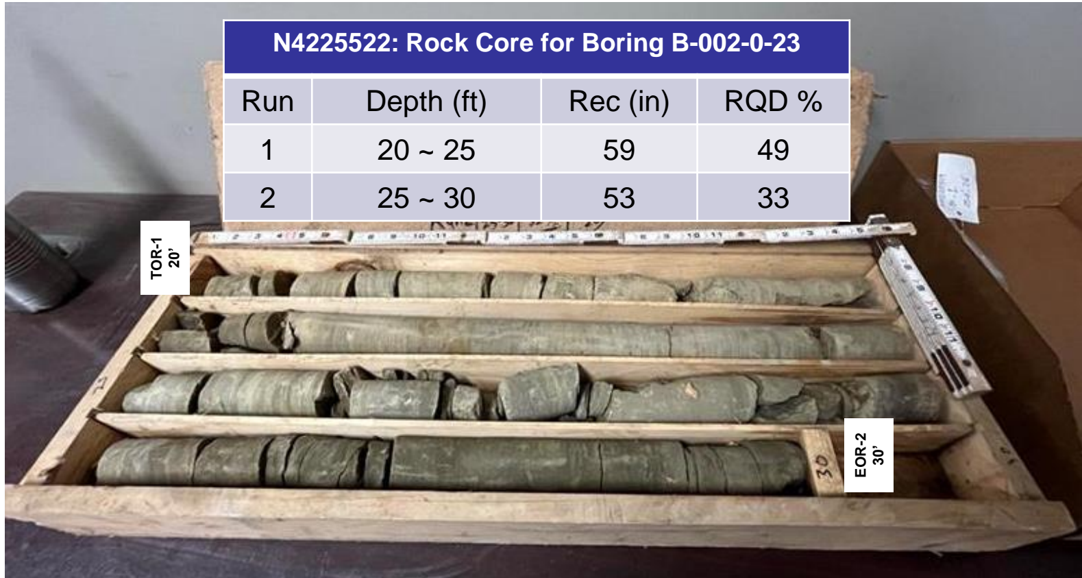
PHOTO 2: ROCK CORE OF BORING B-002-0-23, BOX 1 of 1
